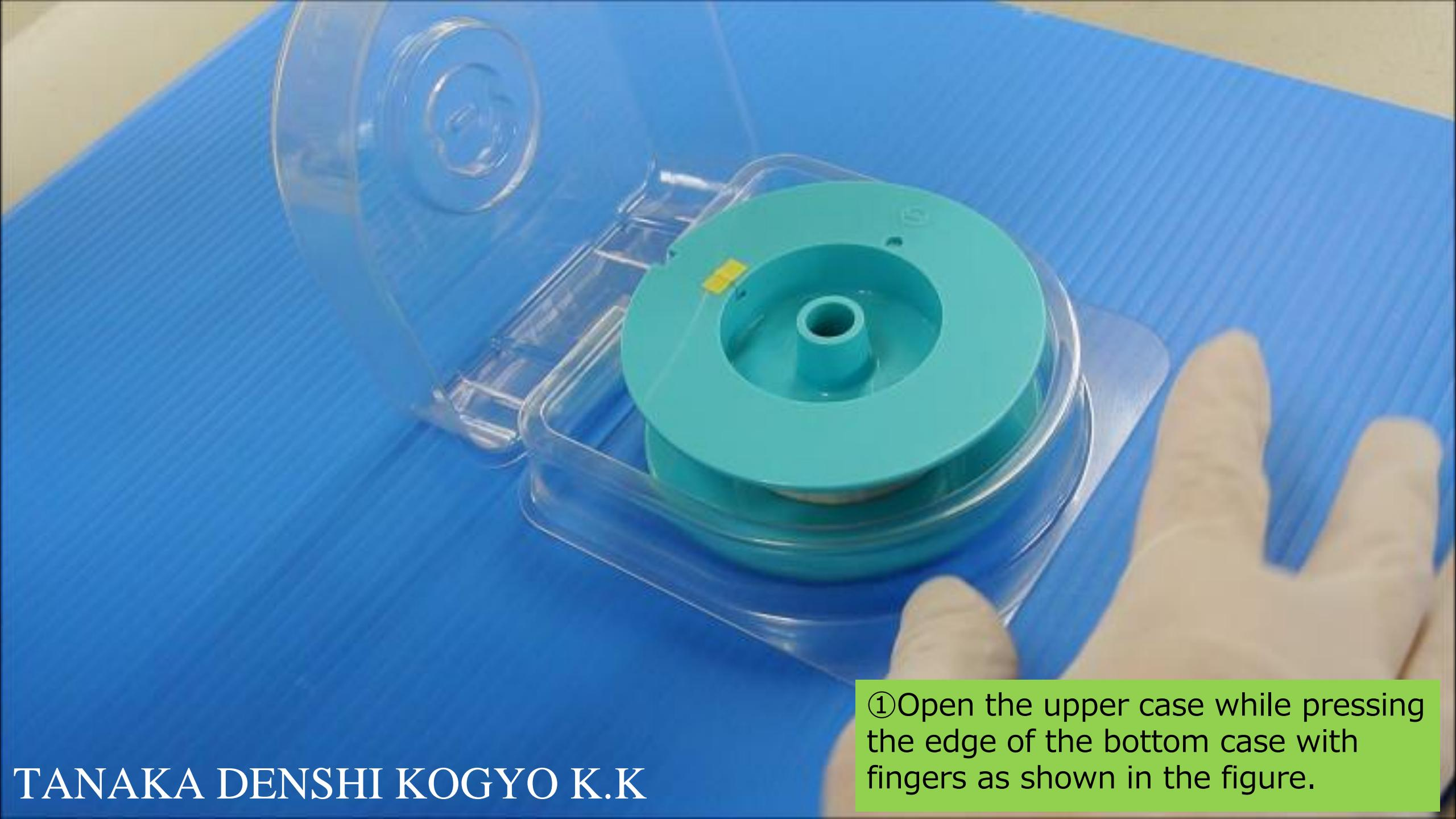
①Open the upper case while pressing the edge of the bottom case with fingers as shown in the figure.
