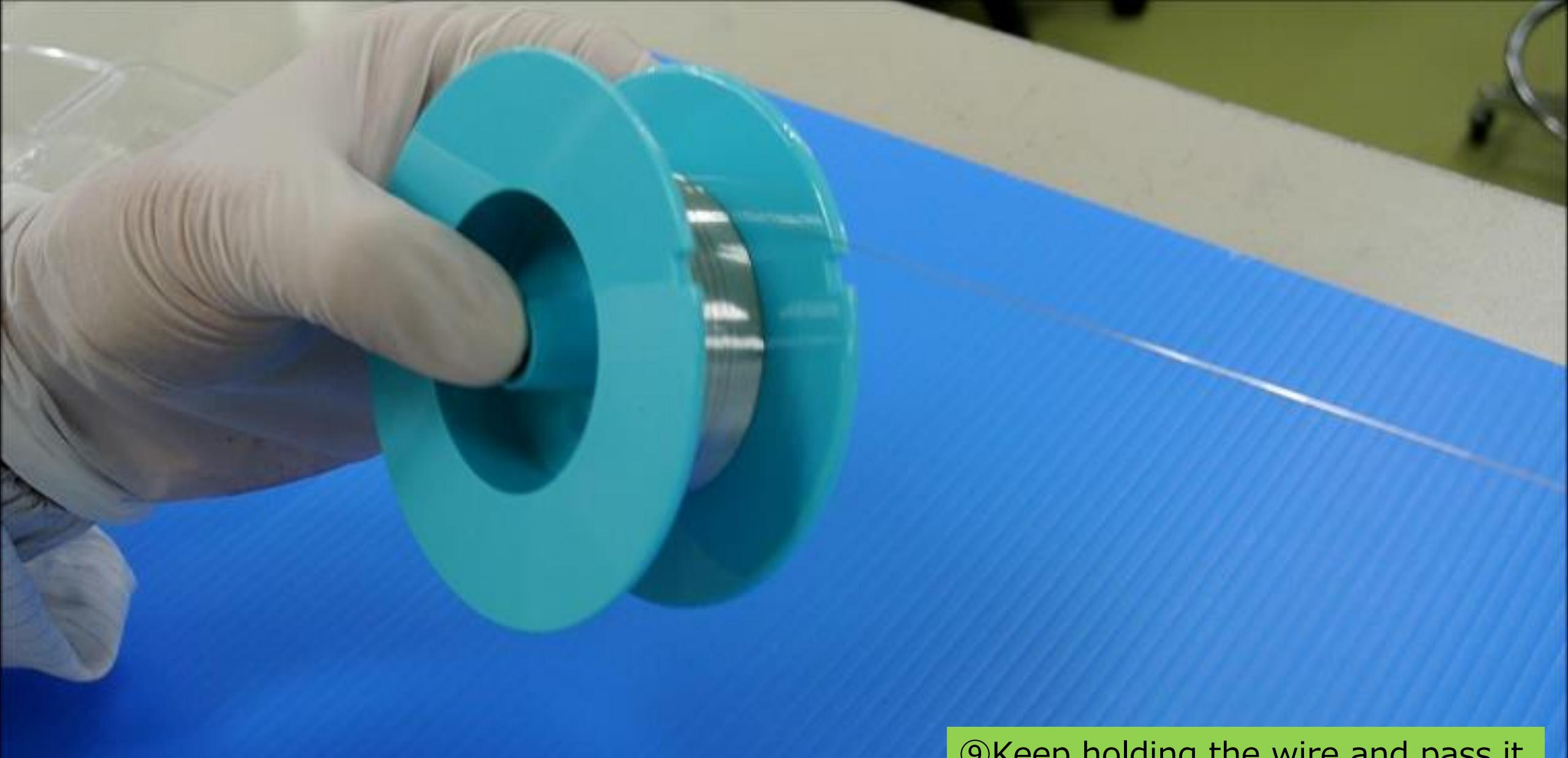
⑨Keep holding the wire and pass it slowly through the notch on the opposite side of the flange.
