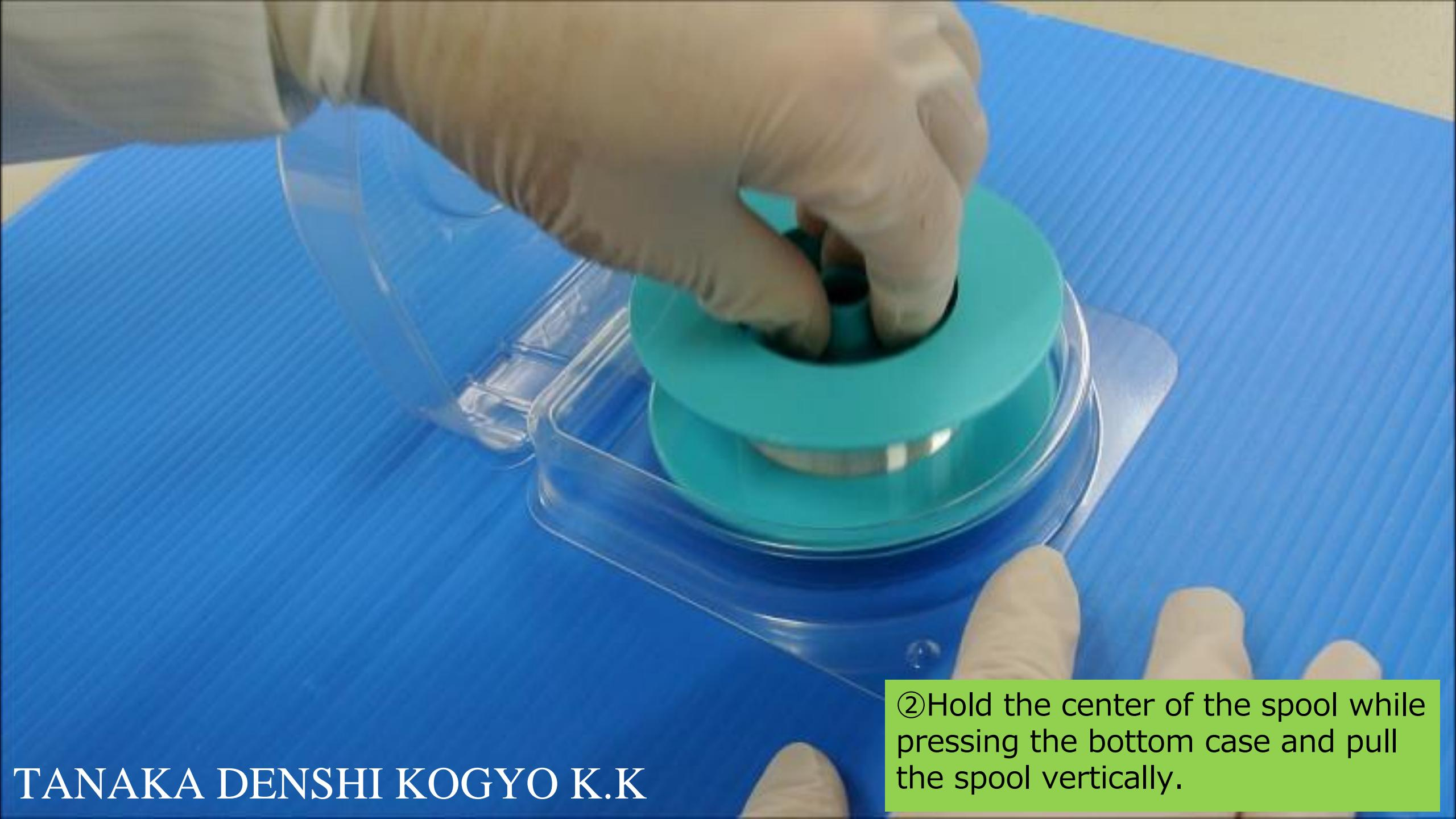
②Hold the center of the spool while pressing the bottom case and pull the spool vertically.
