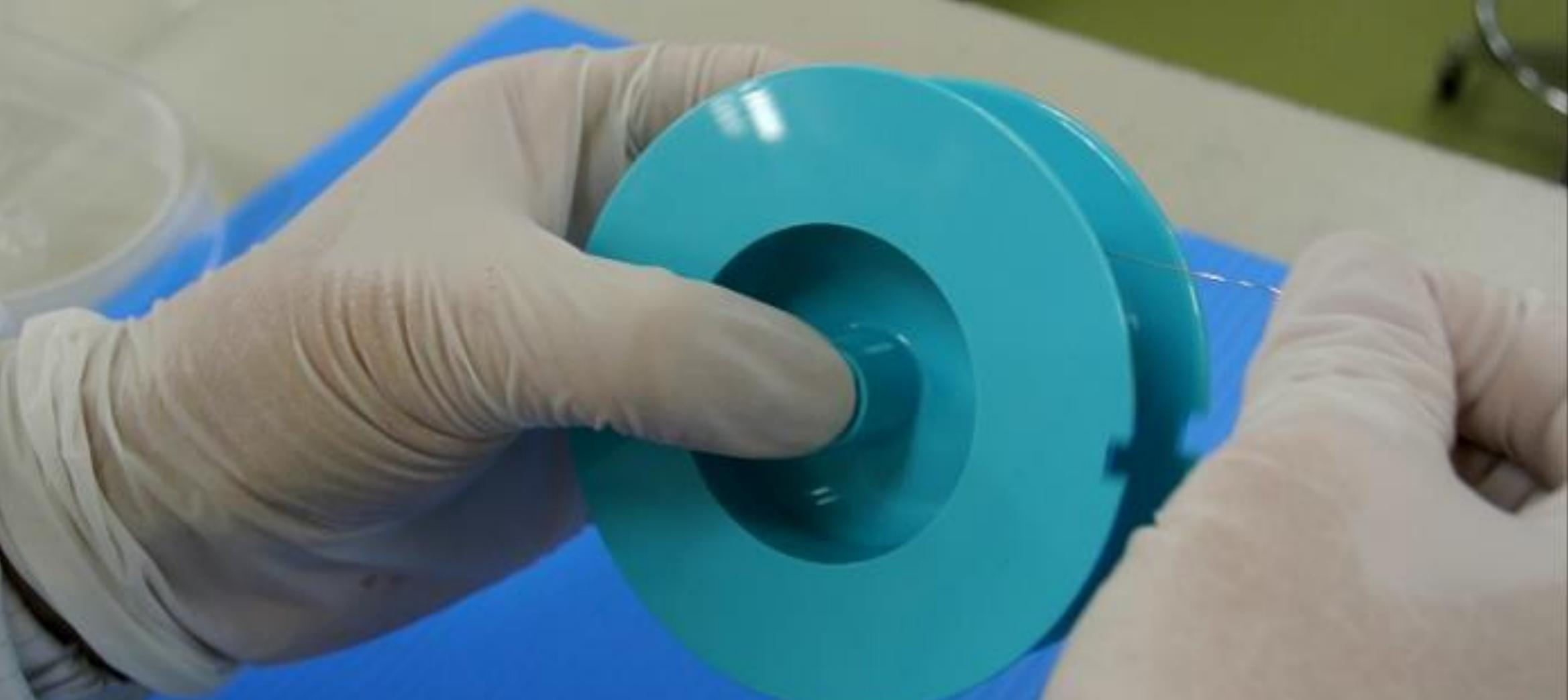
⑧Hold the wire and rotate the spool slowly to unwind it.
