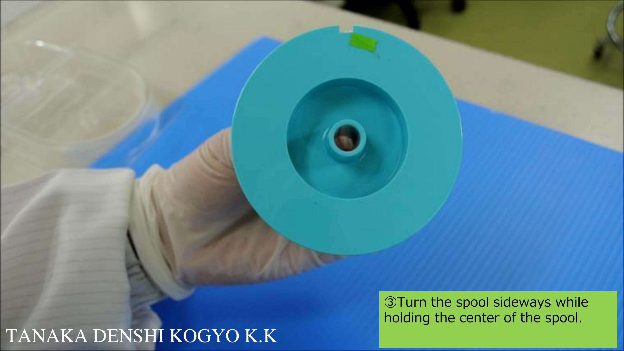
③Turn the spool sideways while holding the center of the spool.
