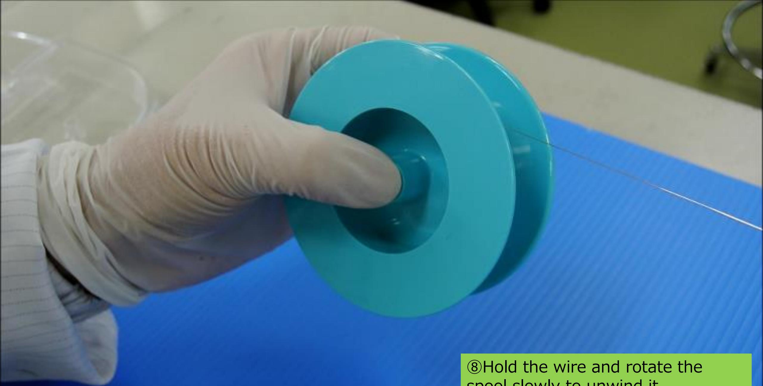
⑧Hold the wire and rotate the spool slowly to unwind it.
