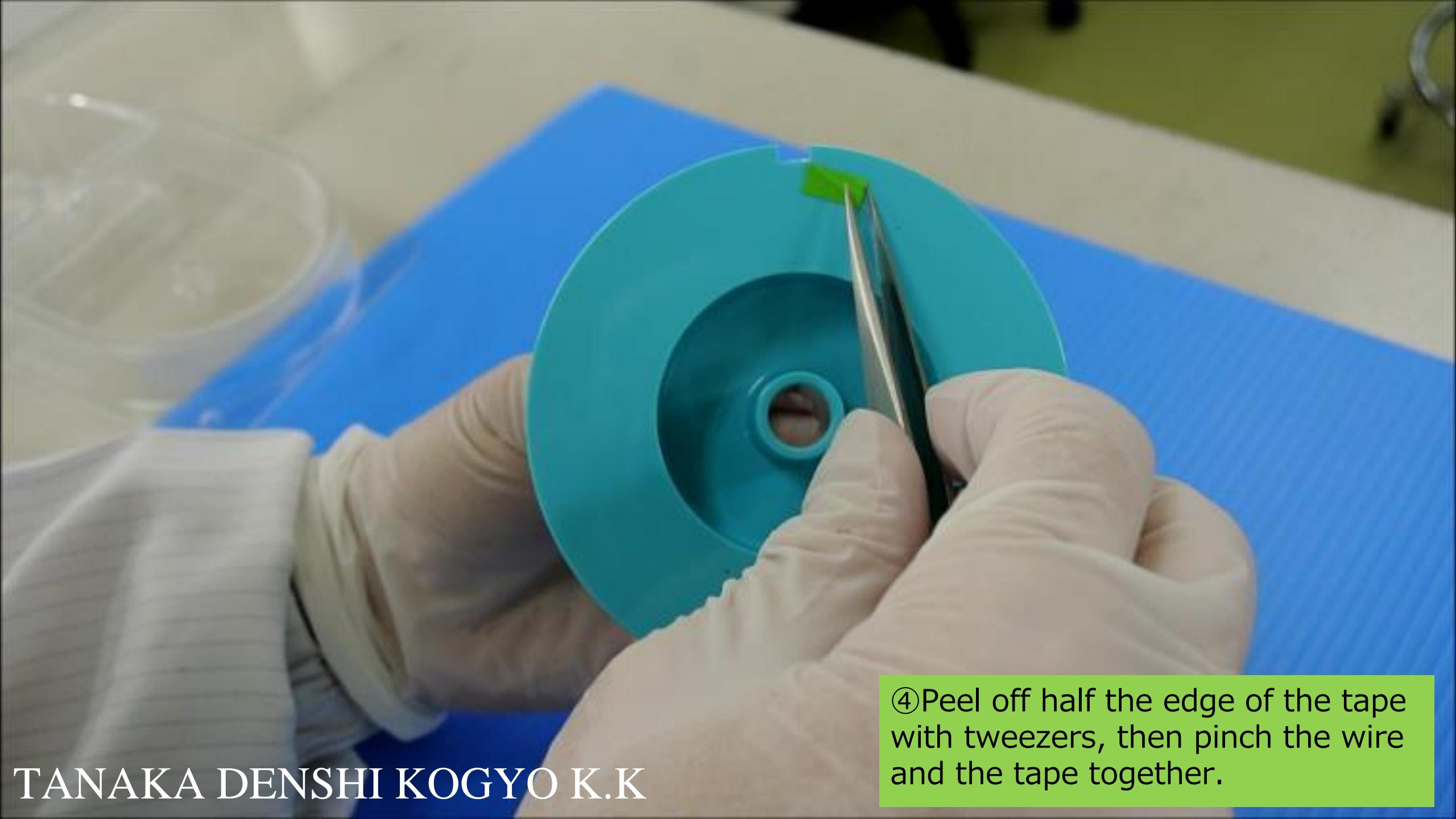
④Peel off half the edge of the tape with tweezers, then pinch the wire and the tape together.
