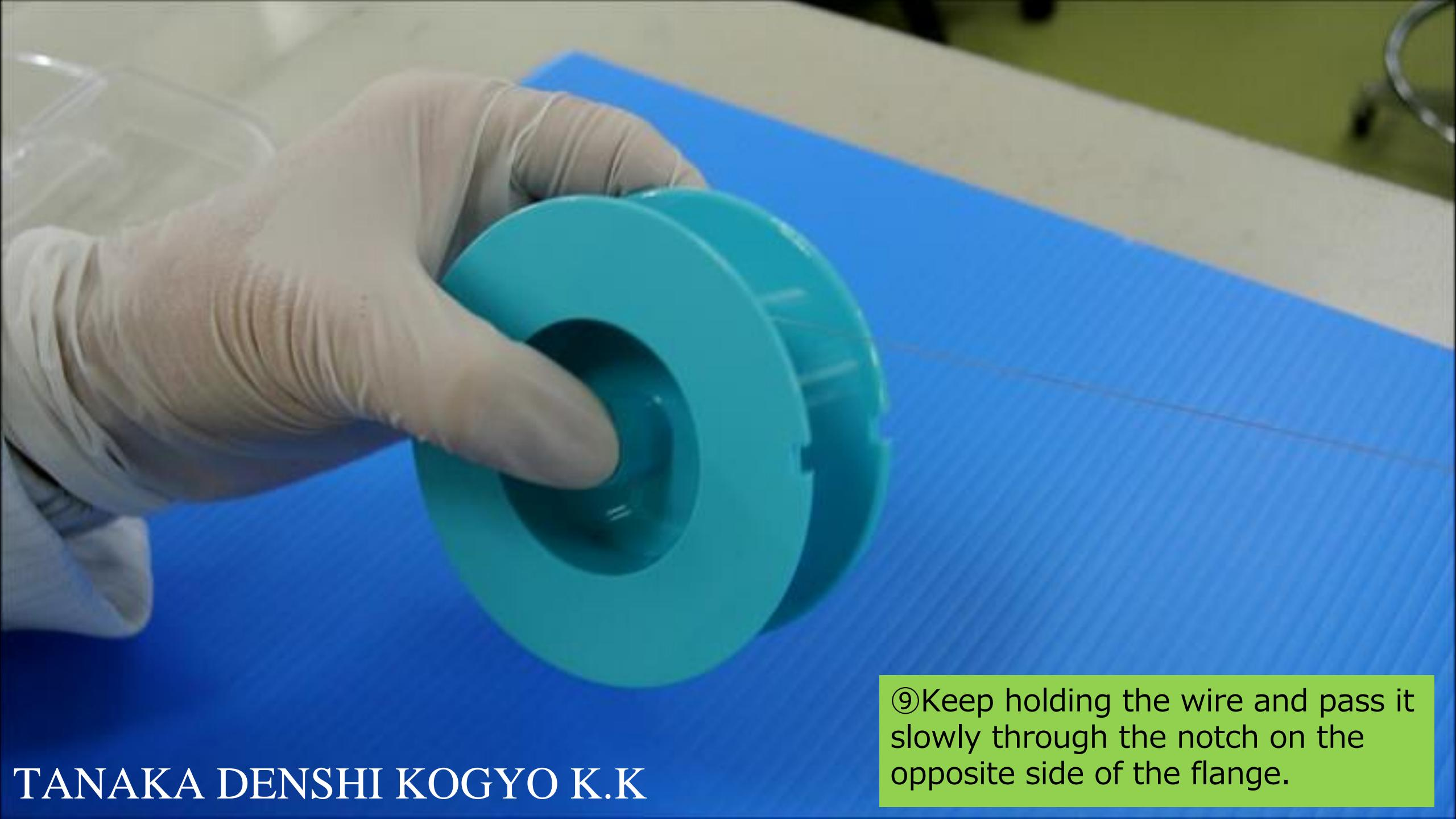
⑨Keep holding the wire and pass it slowly through the notch on the opposite side of the flange.
