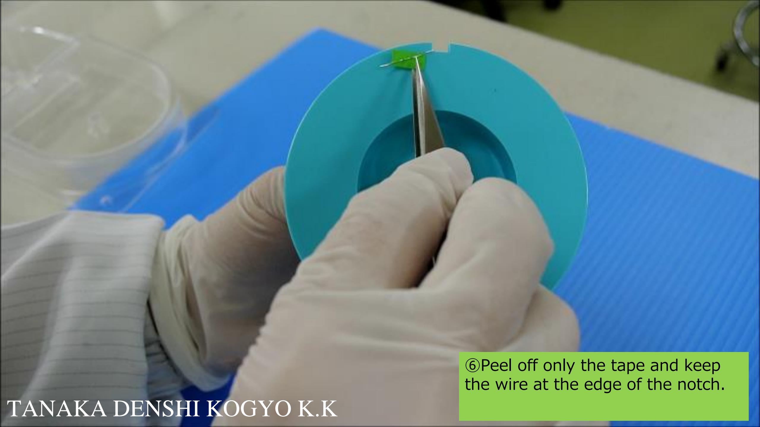
⑥Peel off only the tape and keep the wire at the edge of the notch.
