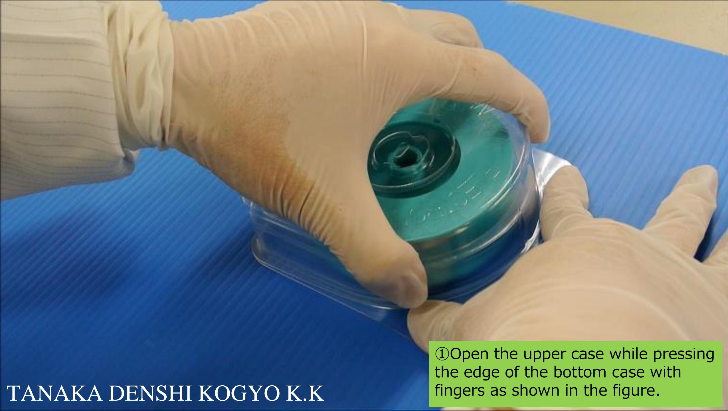
①Open the upper case while pressing the edge of the bottom case with fingers as shown in the figure.
