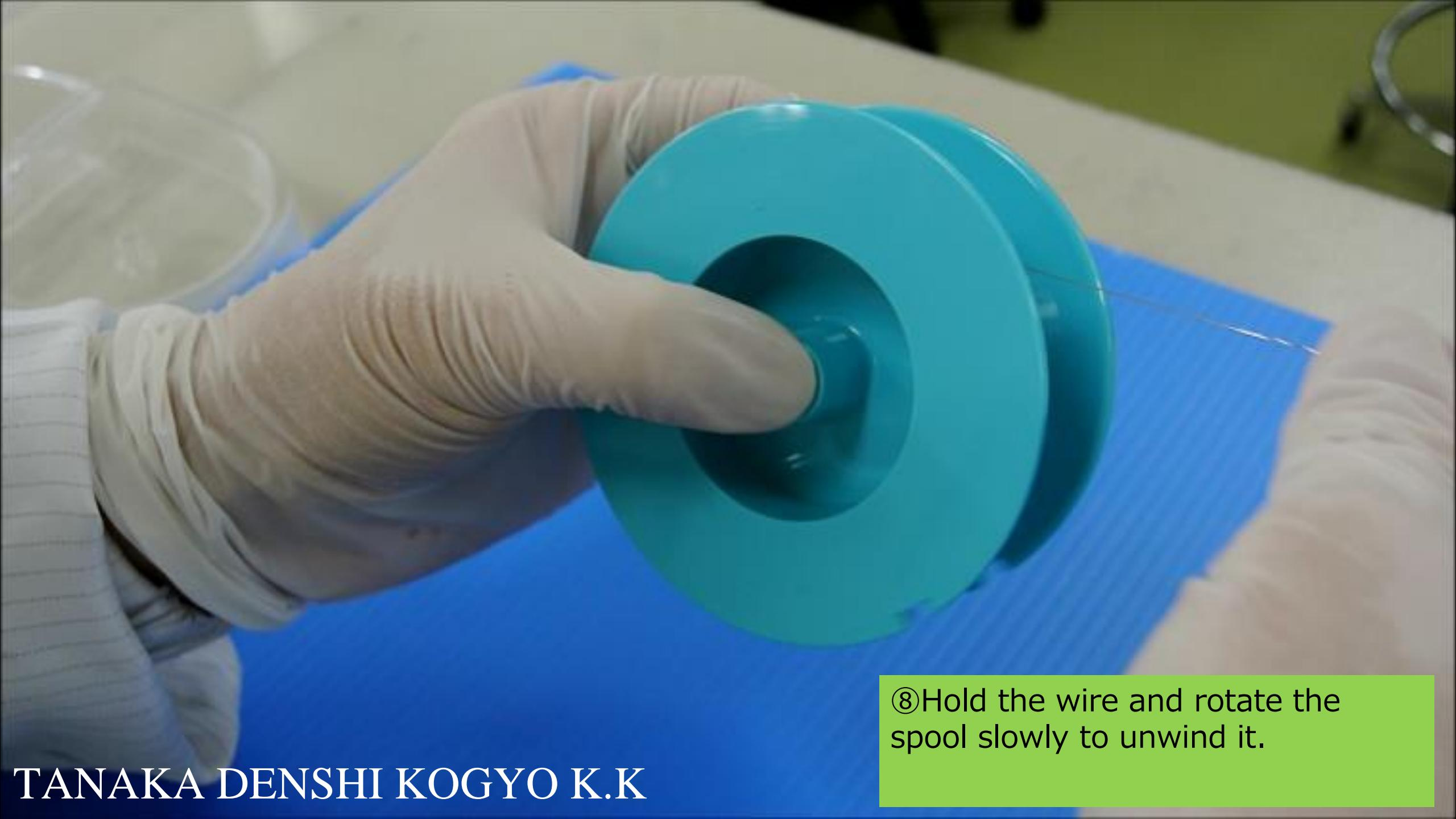
⑧Hold the wire and rotate the spool slowly to unwind it.
