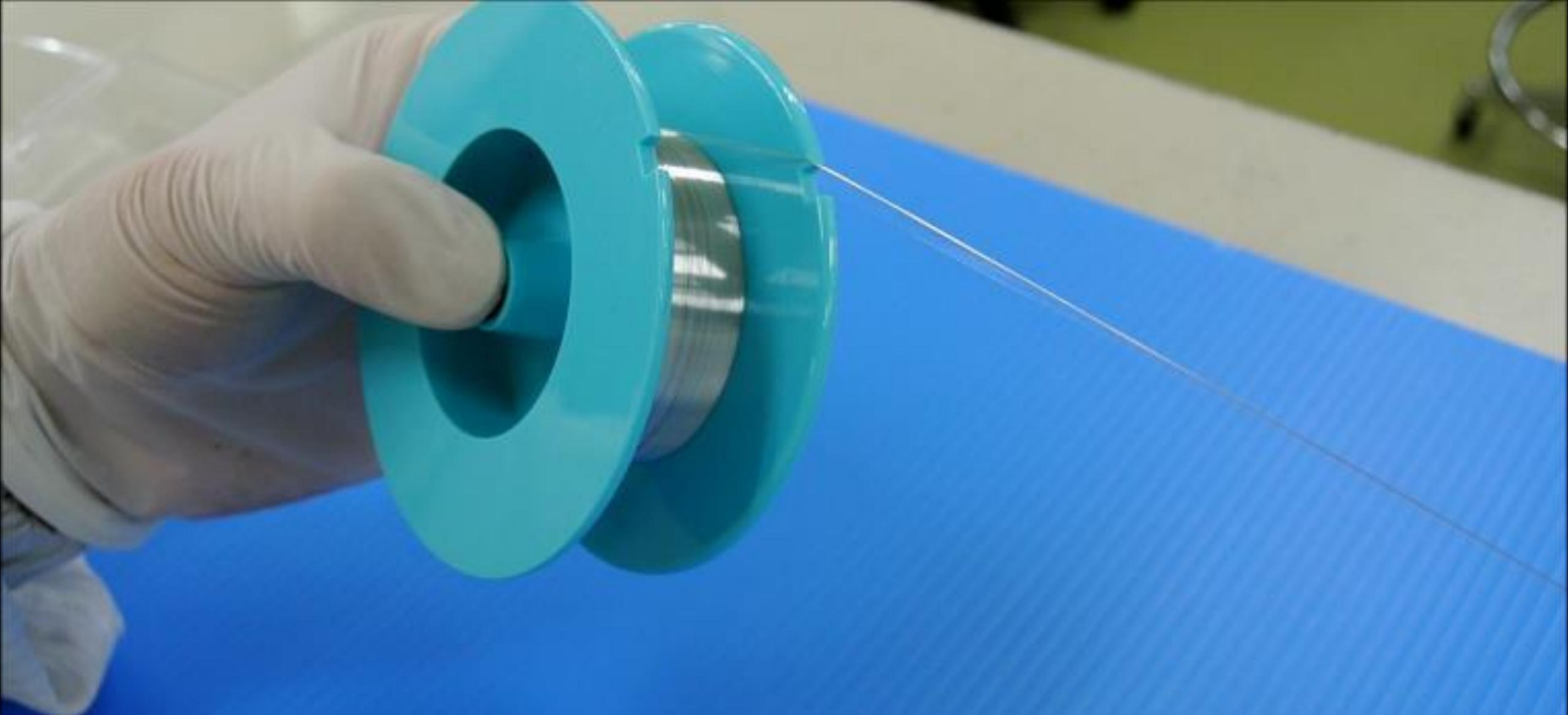
⑨Keep holding the wire and pass it slowly through the notch on the opposite side of the flange.
